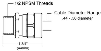
Connector to secures and seal feed cord.
