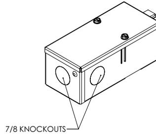
Replaces feed cable for areas where flexible cord cannot be used to bring input DMX signal and 120-277 line voltage power to right end of beginning of run. Box allows 1/2" NPT conduit fitting connection and area for building wire splice connections. Supplied with termination/sealing cap.
