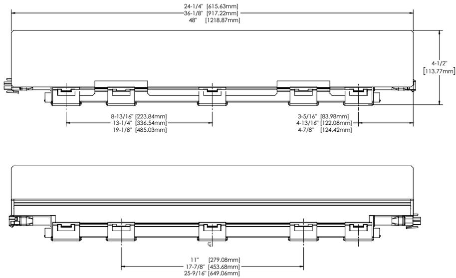
\*The (3) visor clips can also be used for mounting fixture to surface.
