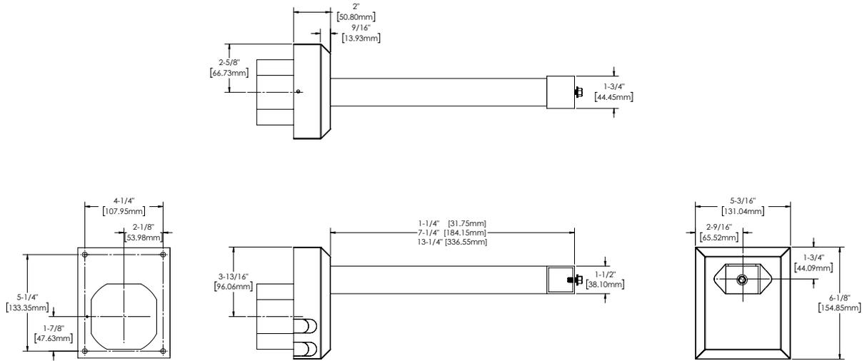
**Cantilever Bracket Detail with M50ADJH2 and Fixture**
