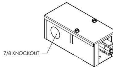
Replaces feed cable for areas where flexible cord cannot be used to bring input DMX signal and 120-277 line voltage power to right end of beginning of run. Box allows 1/2" NPT conduit fitting connection and area for building wire splice connections. Supplied with termination/sealing cap.
