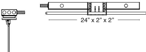
**NOTE:** Multiple drivers must be mounted no less than four inches apart side-by-side, and one inch apart end-to-end, to prevent overheating.
