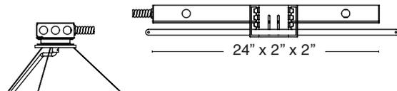
**EM** – Emergency. T-bar install shown, below. Battery pack provides 10W for 90 minutes. Remote install only. Red driver light and test switch mounted in handy box installed at ceiling.
