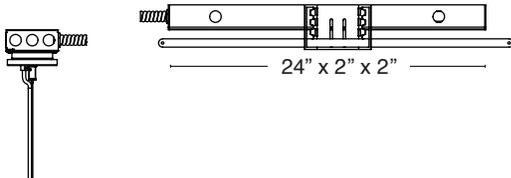
**NOTE:** Multiple drivers must be mounted no less than four inches apart side-by-side, and one inch apart end-to-end, to prevent overheating.
