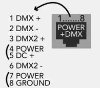
**\*\*CHECK PIN CONFIGURATIONS. APPLYING POWER TO THE DMX INPUT WILL DAMAGE THE CONTROLLER\*\***
