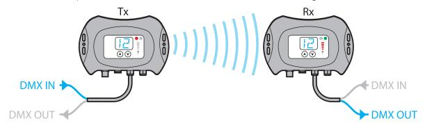
No configuration changes are required to change between operation as a transmitter or receiver; the detection of a valid DMX input will automatically prompt an Aria unit to become a transmitter.
