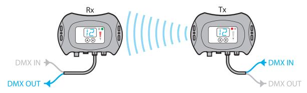
Up to 250 Aria units (or Aria Direct Connect compatible lighting fixtures) can act as receivers from a single Aria transmitter:
