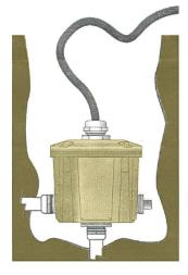
Seal threads. Tighten locking screw on bottom of cover. Connect all wires observing polarity (ie. green-to-ground, white-to-common, and black-to-voltage). Comes with 1/2° strain relief.
