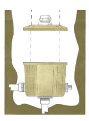
Connect brass junction box to conduit system. Seal conduit entries inside junction box with a good grade RTV sealant per sealant manufacturer's instructions. Note: Drainage must be inplace below junction box. STEP 3:
