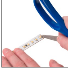
Scrape protective coating from contacts
