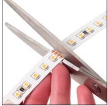
Cut in middle of joining contacts
