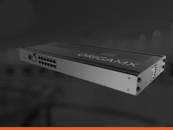
The OrigamX Hub empowers electricians and contractors to provide power and data to remotely located OrigamX Modules for clean and simple installations in architectural, museum, and entertainment applications. Capable of powering and controlling up to 12 Modules, the OrigamX Hub utilizes a common CAT5e cable to deliver both low-voltage power and DMX signal to a Module located up to 240' (73m) away from the Hub.
