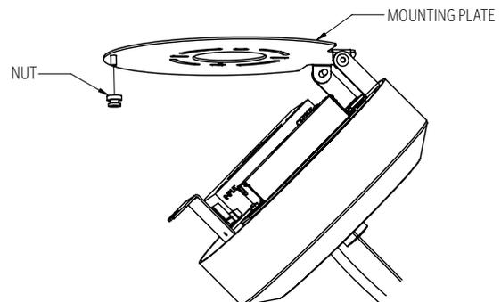
**PIFG** PENDANT WITH 5" FLAT CANOPY, SINGLE CENTER AIRCRAFT CABLE AND WHITE POWER CORD; MOUNTS TO 4X4 OCTAGON J-BOX (BY OTHERS); REMOTE DRIVER ENCLOSURE: **NOTE: REQUIRED FOR DM8, DALI, OR DMX CONTROL**
