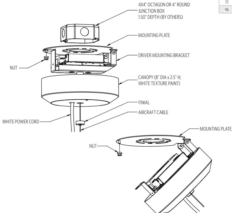
**PIFG** PENDANT WITH 5" FLAT CANOPY, SINGLE CENTER AIRCRAFT CABLE AND WHITE POWER CORD; MOUNTS TO 4X4 OCTAGON J-BOX (BY OTHERS); REMOTE DRIVER ENCLOSURE; **NOTE: REQUIRED FOR DM8, DALI, OR DMX CONTROL**
