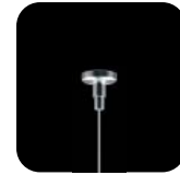
4" diameter machined power feed and 1-1/4" diameter machined non-power feed canopy. Offers minimal ceiling treatment while maintaining the ability to cover mistakes. Requires a 1/4-20 stud securely fastened to the ceiling.
