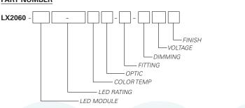
Example Part Number: **LX2060-L1915-90DWM9-CT1-DX120W** is a fixture with a Lumenetix-araya 19mm LED module, 1500 Lumen/90 CRI/29 Watt LED rating, Dynamic White (1650° - 8000°K) Color Temperature, 70mm 20° Optic, CT1 CONTROLTrack fitting with DMX Address knobs and DMX compatible control gear, 120V and a White finish.
