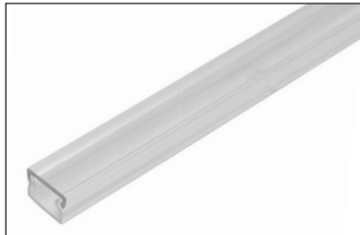
DL-O-2PC-C (Clear) DL-O-2PC-F10/F30/F60 (Frosted) Two-piece mounting tube; base (clear) with cover, sold in 4 foot lengths. Used with Duratape (no PVC sleeve) for linear applications. Clear or frosted at 3 diffusion levels, 10%, 30% or 60%.
