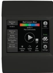
**Easyl™ Solo:** Is a standalone entry-level controller enabling show creation and playback directly at the LCD touchscreen.
