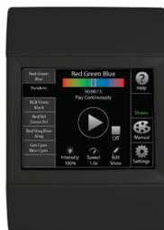
**Easyl™ Solo:** Is a standalone entry-level controller enabling show creation and playback directly at the LCD touchscreen.
