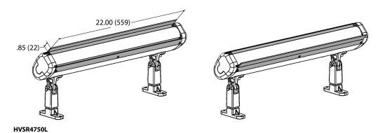
**HALF VISOR** are factory installed on top side except for wall wash distribution which is installed on the bottom. Visors: Can be field installed and moved from top to bottom if desired.
