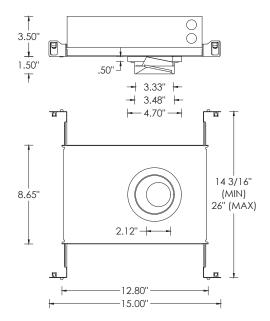
**NC** - New Construction Housing (Non-IC and CP rated) **IC** - New Construction IC Housing (2200lm max)
