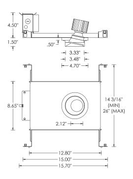
SH - Shallow Housing (IC and Chicago Plenum Rated) (2200lm max)
