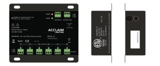
The **RDS 6** is a RDM/DMX splitter and optimizer. It features one RDM/DMX input and six outputs, allowing for flexible configuration of your RDM/DMX signal. Each port is electrically isolated to ensure you get the maximum total run of 3,900' for each signal line.
