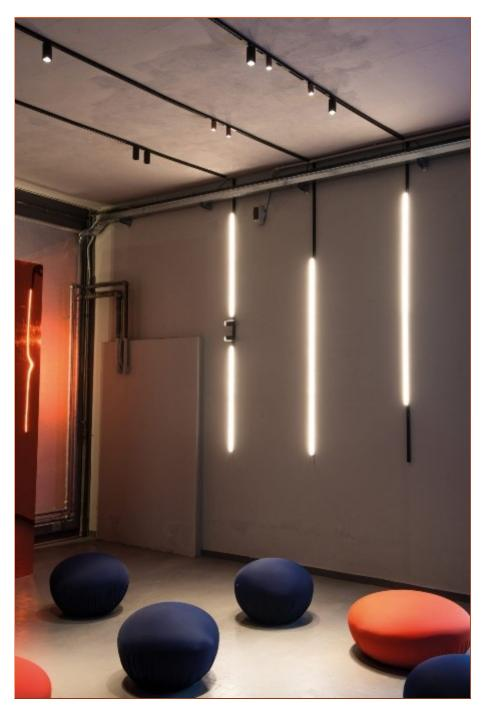
Targetti FORTYEIGHT LABEL projectors are available in three sizes. Specially designed for applications in the retail, interior and hotel sectors with a simple, minimal shape and small dimensions. All versions utilize remote power supplies to minimize visual impact. A new range with a miniaturized LABEL 2 (Ø0.79"), LABEL 4 (Ø1.57") and LABEL 6 (Ø2.32"), all equipped with Ra90 LED sources and professional performance.
