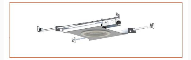
Amico LP6 MRI Downlight: The non-ferrous LP6 light fixture is designed for MRI suite applications. It can be mounted directly into a dry wall ceiling or a suspended ceiling grid using the optional Suspended Ceiling Mounting Bracket Assembly. The LP6 Contains no on-board electronics therefore will not interfere with MRI imaging. With a total depth of 2 3/8", the low profile form factor allows for installation in even the most crowded of plenum spaces.
